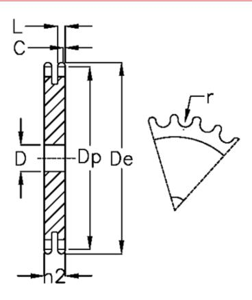
C = 2 D = 25 De = 255.2 Dp = 247.78 For chain size =  $5/8 \times 3/8$ For chain type = 10 B-2 h2 = 25.5
